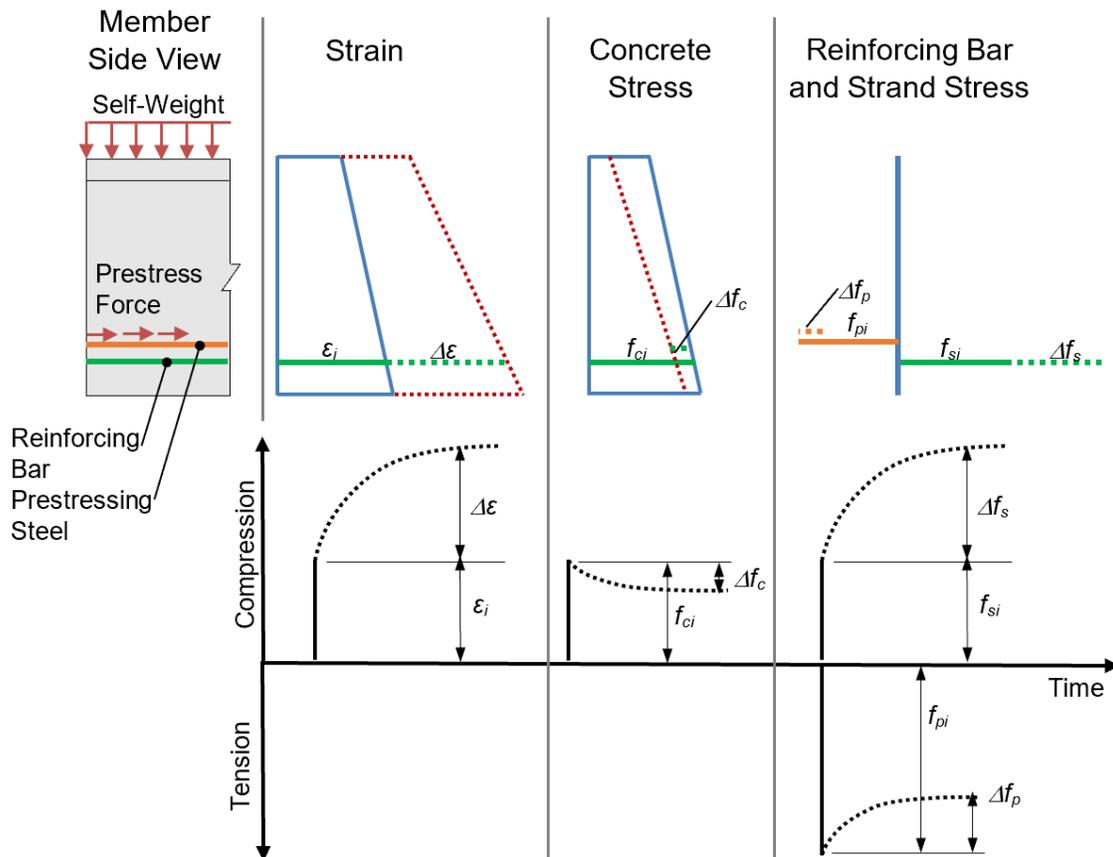
**Figure 3**— Time-dependent effects in prestressed member with non-prestressed reinforcement.  $\varepsilon$  = strain,  $f$  = stress,  $x_c$  = concrete,  $x_s$  = non-prestressing reinforcement,  $x_p$  = prestressing steel,  $x_i$  = initial condition,  $\Delta$  = change over time
