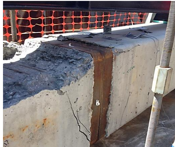
Fig. 10 – Failure of compression zone of Test 1 (left) and Test 2 (right)
