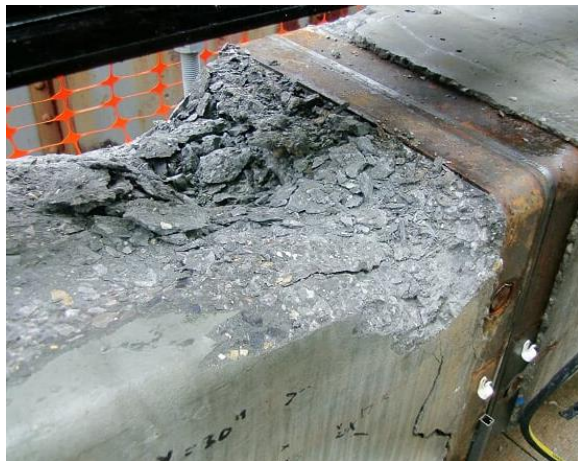
Fig. 10 – Failure of compression zone of Test 1 (left) and Test 2 (right)
