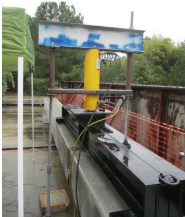
Fig. 8 – Hydraulic jack and spreader beam
